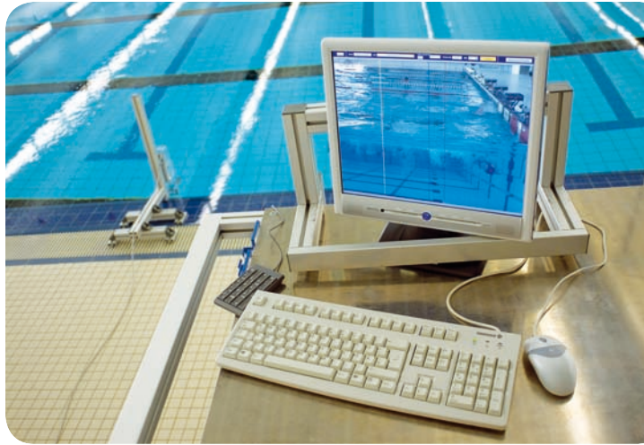
Fig. 27: New analysis set-up for starts and turns. Four digital high-speed cameras monitor the athletes during their performance. One of the two underwater cameras can be seen in the background
